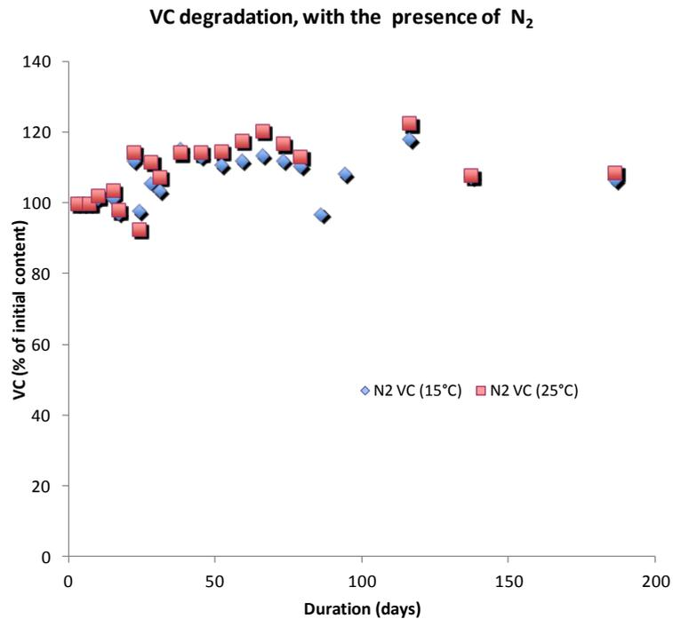
Figure 12 : Degradation of VC observed during 186 days for the microcosm incubated at 25°C and 15°C with N<sub>2</sub>
