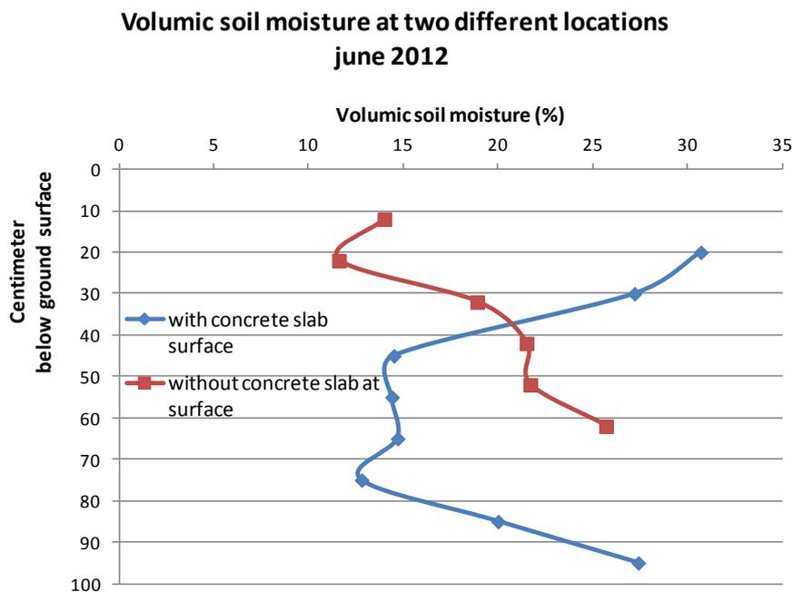
Figure 8 : Volumetric soil moisture for two locations (near the piezometer Pz 3)
