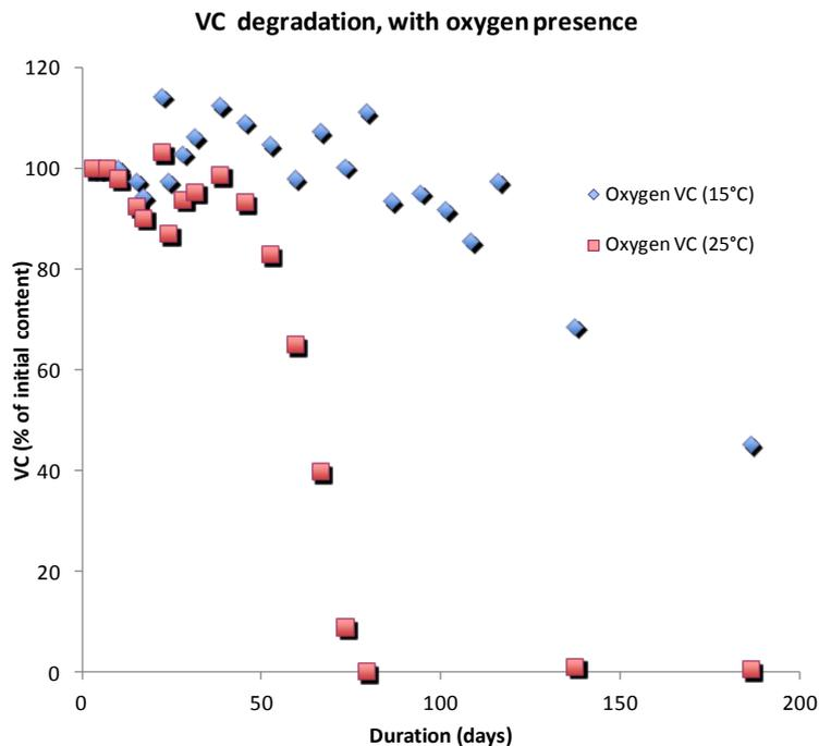
Figure 10 : Degradation of VC observed during 186 days for the microcosm incubated at 25°C and 15°C with oxygen presence
