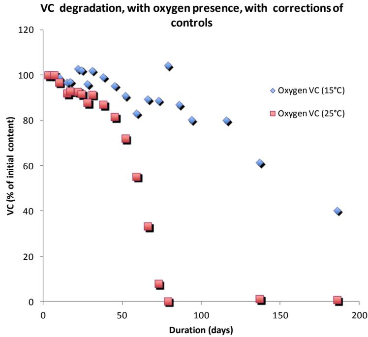
Figure 11 : Degradation of VC observed during 186 days for the microcosm incubated at 25°C and 15°C with oxygen presence, with controls corrections.
