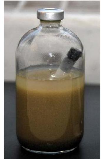
Figure 4 : On the left, VC degradation with very low concentrations of dissolved oxygen (Gossett & al., 2010), and on the right is an example of a microcosm saturated with permeation tube.
