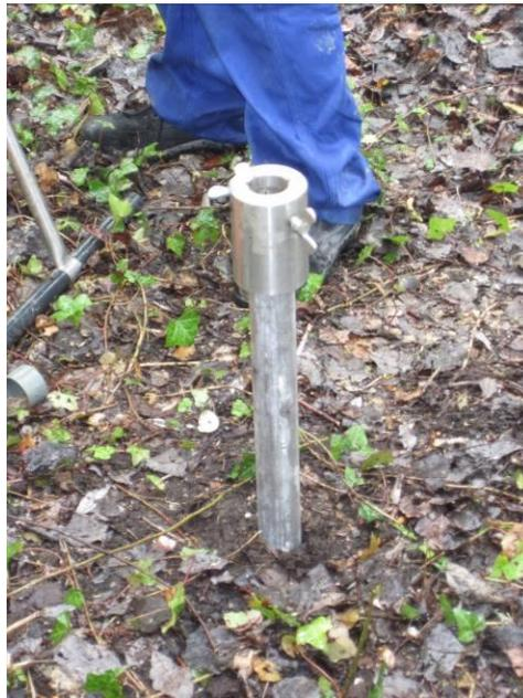
Figure 5 : Specific tube used for the TDR measurements
