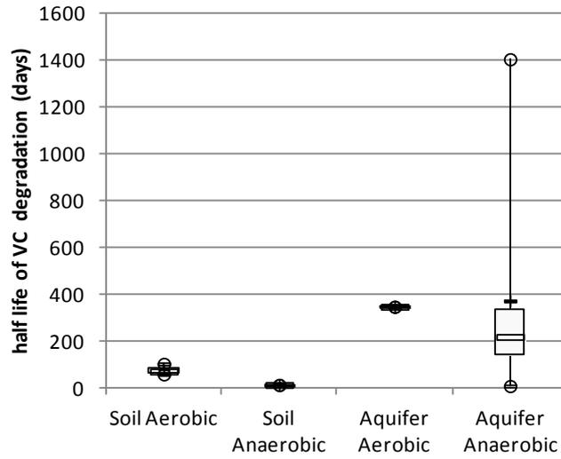
Figure 14 : Box plot of half life VC degradation for the 2 types of soil and 2 types of redox conditions
