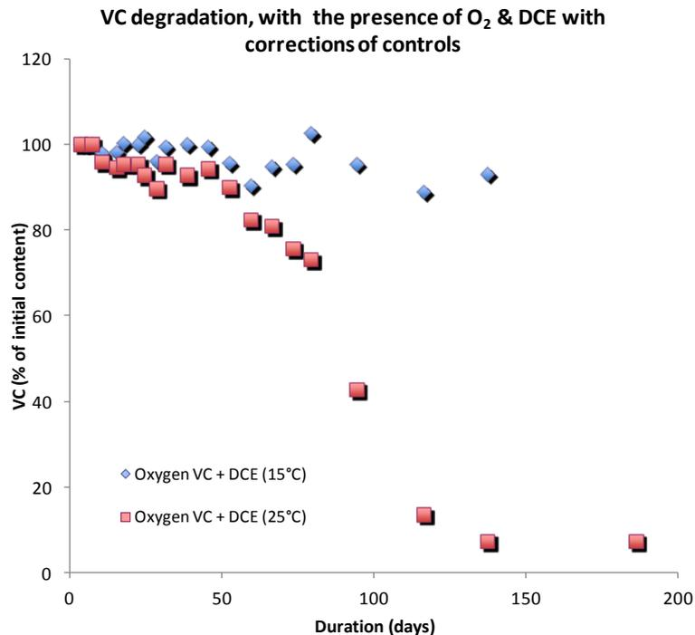
Figure 13 : Degradation of VC observed during 186 days for the microcosm incubated at 25°C and 15°C with N<sub>2</sub> and c-1,2-DCE
