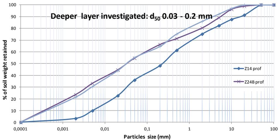
Figure 9 : Uniform distribution of the particles sizes of the deeper layer investigated by auger
