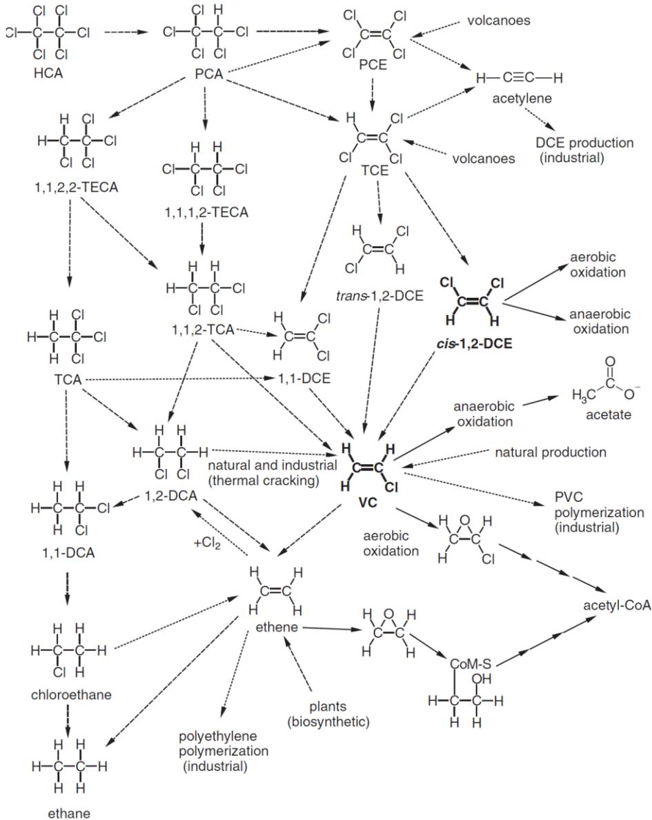
Figure 3 : Metabolic degradation of chlorinated ethanes and ethenes by Mattes (2010). The arrows indicate the oxidative biological reaction, the dashed lines indicate reductive biological reactions, and dotted lines indicate abiotic reactions
