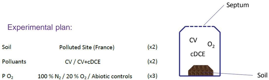
Figure 6 : Experimental plan used for the laboratory microcosms
