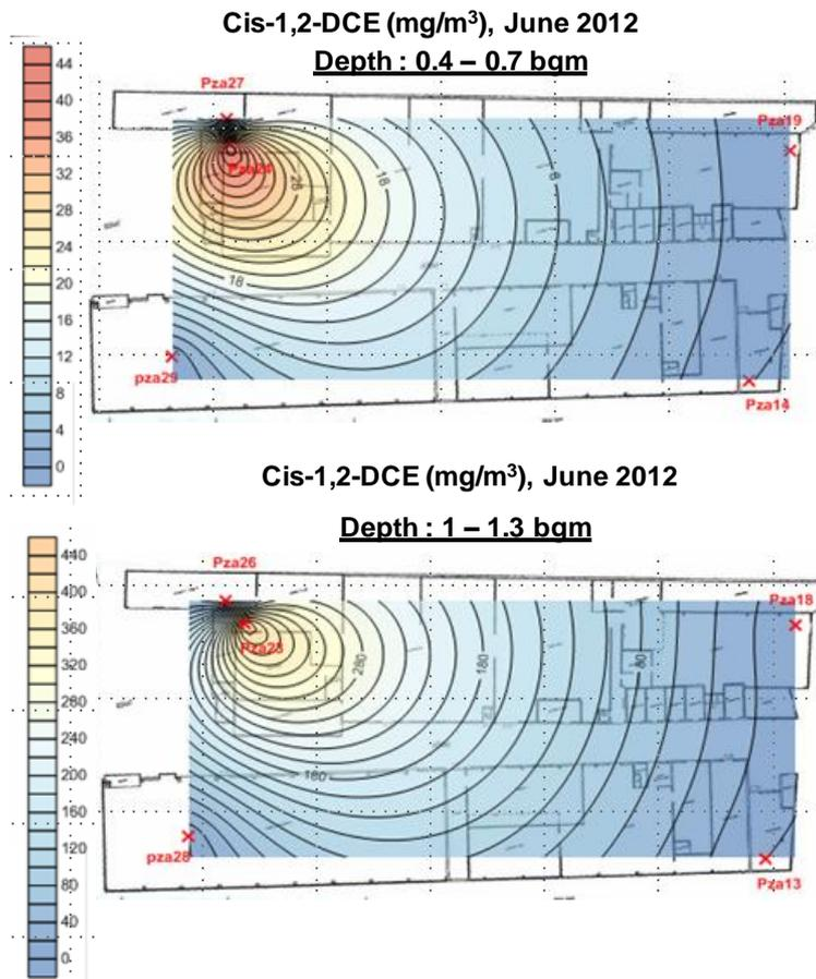
Figure 2 :Cis-1,2-DCE gas soil concentration by active sampling at two depth (June 2012)
