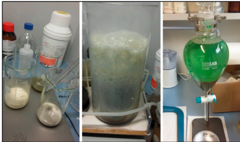
Figure 7 Example set-ups for degradation (left and centre) and density separation (right) for the removal of organic and inorganic components. Image taken from source (Campanale C., 2020).
