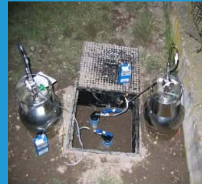
Summa-Canister (6 L, suction rod and veriflow system) (source: INERIS)
