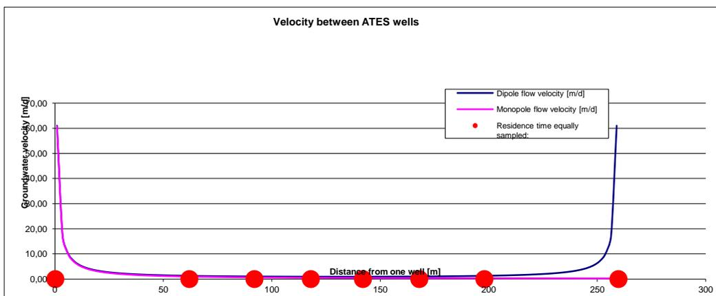
Figure 1: Steady state velocity distribution between the two wells and observation points located at distances separated by equal travel time.
