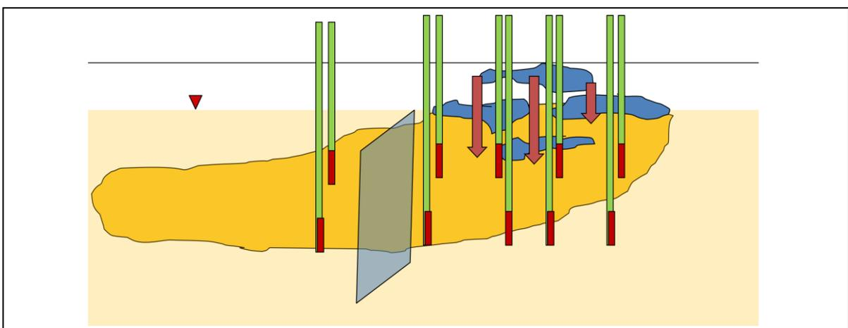
Figure 4: Schematic representation of the positioning of samplers to determine the flux.
