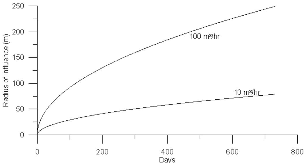
**Figure 9: Calculated radius of influence for 2 continuous pumping rates over a 2 year period**
