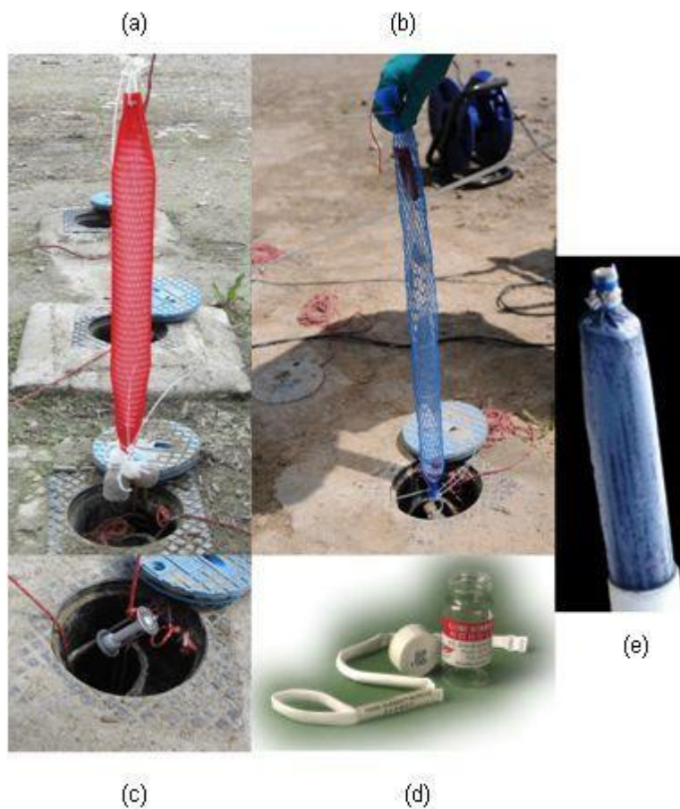
Figure 3: Passive samplers tested in the frame of the CityChlor project (a) PDB; (b) Regenerated cellulose dialysis membrane; (c) Ceramic dosimeter (d) Gore® sorber module; (e) PFM
