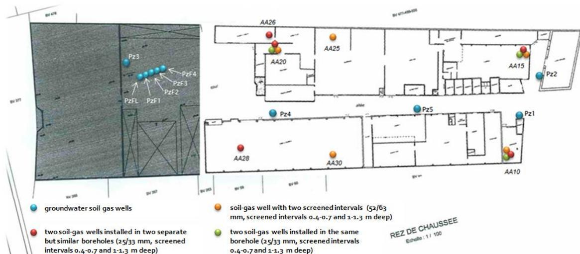
Figure 1 : Description of the site and of the location of the piezometer (Pz1 – Pz5) and of the locations of the soil gas wells.
