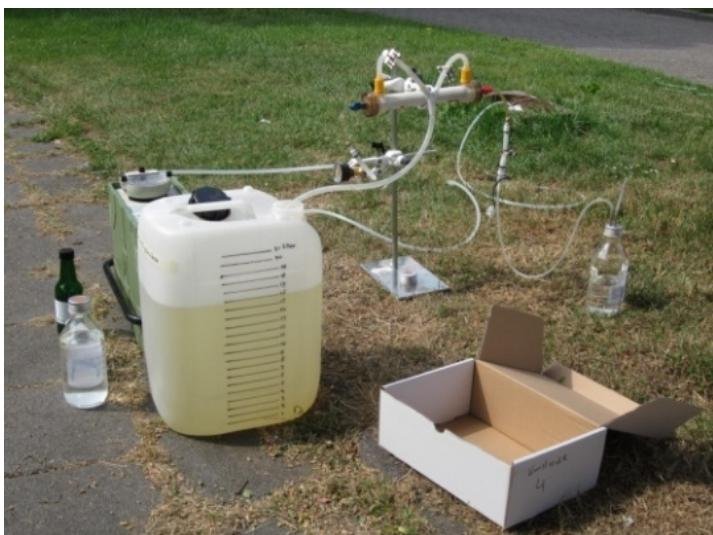
**Figure 4** Sampling using the dialyser method
